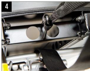
rail hinge or around the gas struts. **STEP 6.** Push the glideboard to the desired upper motion limit and hold it there. Then pull the end of the strap from the buckle until there is no slack in the buckle loop and strap. Test the motion of the glideboard with your hands. The buckles should hold a firm grip on the straps from the glideboard.
